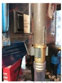
The adaptor will clip into the casefeeder where the normal plastic drop tube connects the Dillon™ casefeeder to the Dillon™ reloading press. The flexible PVC hose supplied will connect the adaptor clip to your rollsizer drop tube.
