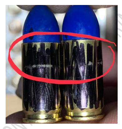
Please note that all reloading presses flex to a degree (even high-end commercial presses when using fired cases). The settings of the reloading press should only be considered final once the shell plate assembly is filled with cases and the press is fully loaded. It is often necessary to adjust the dies further once the shell plate is full of cases. Rollsizing your cases will reduce the load on your reloading press to a significant degree.
