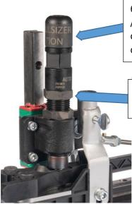
6A. Remove this cap to remove / replace the Guide Rod / decapping pin. It can be difficult the first time.
